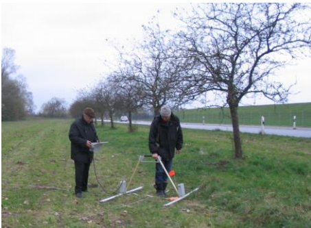
Fig. 4. Field operation with Loza-V GPR.
